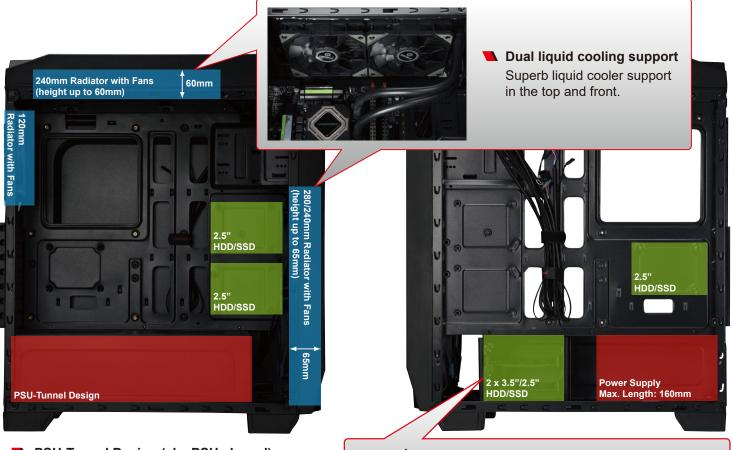
PSU-Tunnel Design (aka PSU shroud)
