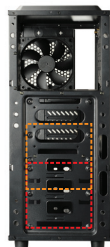
One front 120mm fan support (middle or lower slot)
