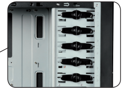
Toolless ODD installation
